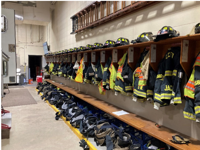
Photo 2 – The storage of turnout gear in the apparatus bay is not consistent with the recommendations of NFPA 1500 for carcinogen mitigation and cancer risk reduction
