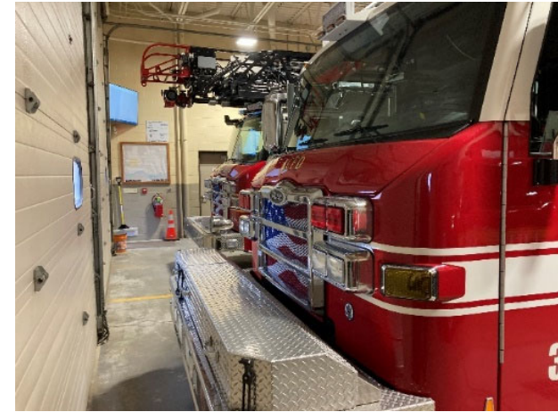
Photo 3 – Apparatus back in and do not provide a safe walking distance between the front of the rig and the overhead doors.
