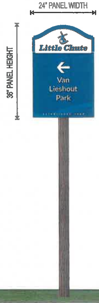
SIGN TYPE F | SMALL DIRECTIONAL ALUMINUM PANEL - PAINTED ONE COLOR DIGITAL PRINT VINYL GRAPHICS SUPPLY PANELS TO CUSTOMER
