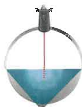
Adaptive Focus Vertical scan for maximum Doppler power 3 inches above and below face point.
